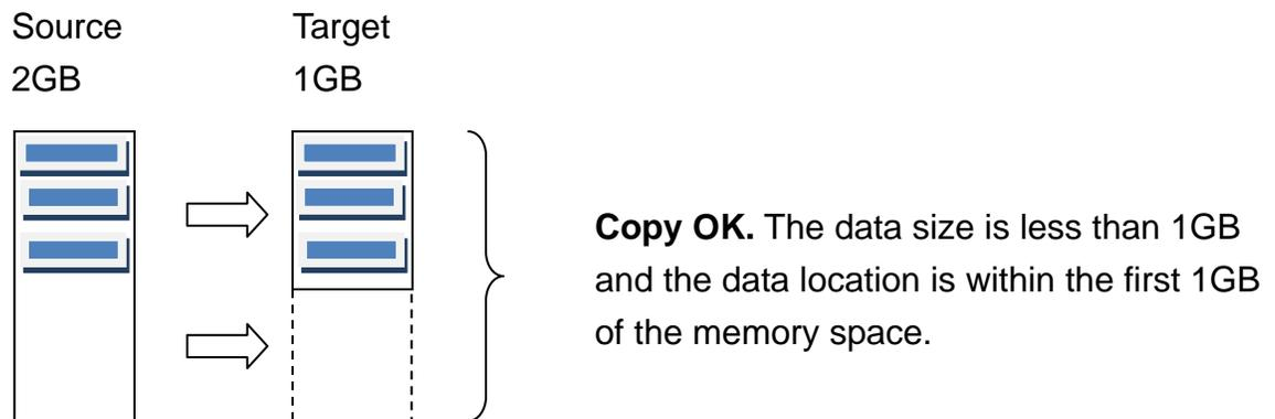
**Illustration 2** For source device with FAT16 or FAT32 file system whose content is located beyond the capacity of target card(s)/ drive(s) while the content size is still within the capacity of the target card(s)/ drive(s) :
