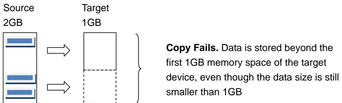
**Illustration 3** For source device with FAT16 or FAT32 file system whose content is located content size is bigger than the capacity of the target card(s)/ drive(s) :
