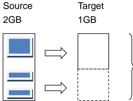
**Copy Fails.** Data size is bigger than the capacity of the target device. Insufficient memory space to complete the copy process.
